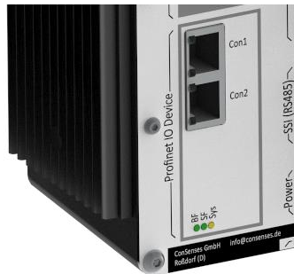
Picture 14: Connectors for the field bus connection
